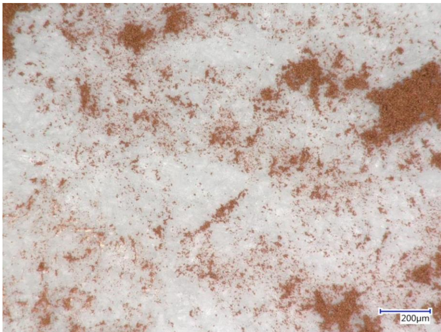
Figure 2: Light microscope image of the "copper powders", x200 These particles are difficult to identify due to super fineness, probably spherical.
